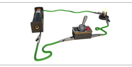
When electricity cannot flow through all the components of a circuit, it is called an incomplete circuit. Loose wires, damaged components and flat cells or batteries can all stop the flow of electricity around a circuit.
